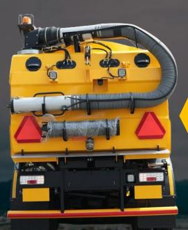
Wander Hose suction hose for cleaning gullies, drain and other awkward areas. Mounted on the Rear Tank Flap. Control extension unit attached Hopper rear door.
